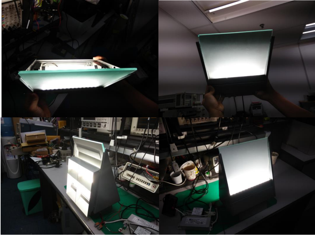
Figure 7: SFO Uplight when turned on using ULE269VW light engine with backlite
